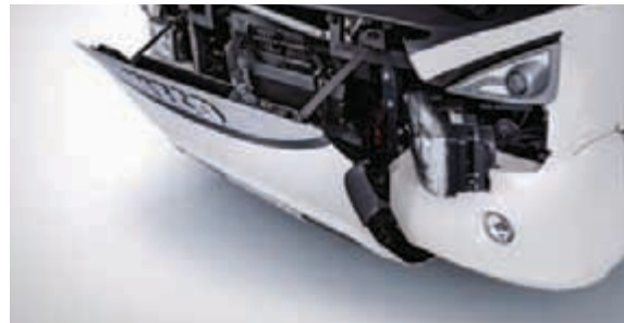
The front grill tilts forwards to enable access to the driver's air conditioning unit and the screenwasher filler. The headlamp housing is pivot-mounted for direct access to wiring and bulbs.
