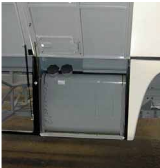
Interurban bus – combined heating fuel oil and diesel tank
