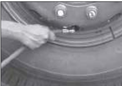
Connecting hose to tyre tube nozzle
