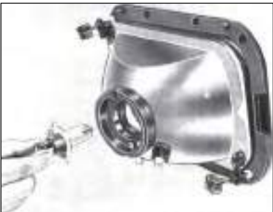
Replacing head lamp bulb
