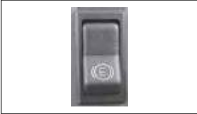
Exhaust brake isolator switch
