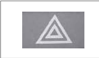
Hazard warning indicator
