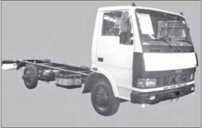
LPT 613 - Full forward control truck with tilt cab (RHS view)
