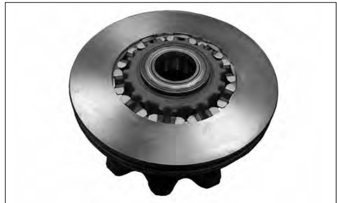
FIGURE 90 - INTERMEDIATE ELEMENTS (SPACERS) INSTALLED
